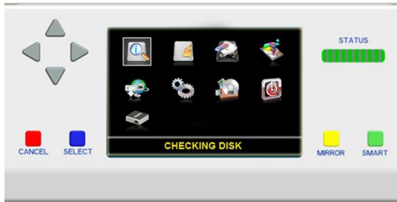
Figure 6: Front Panel with LCD, status LED and control buttons
